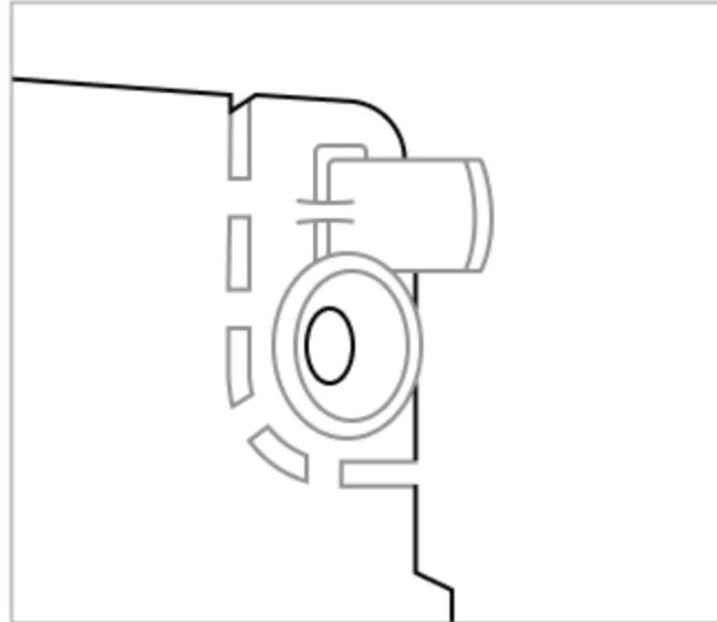
5. Slide KeyPad Plus onto the mounting plate and tighten the mounting screw at the bottom of the body. The screw is needed for more reliable fastening and protection of the keypad from quick dismantling.
